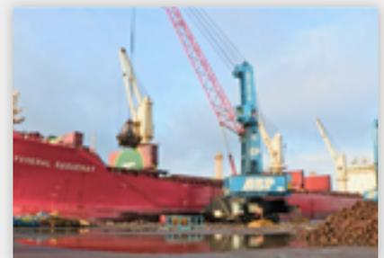
This 280-tonne Gottwald port crane has a lift capacity of upto 100 tonnes
